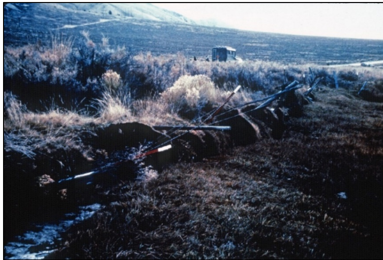
Figure 6-2. Photograph showing buckled and overturned sod at the toe of the lateral spread along Highway 93 at the 1985 Whiskey Springs investigation site (Youd et al. 1985).
