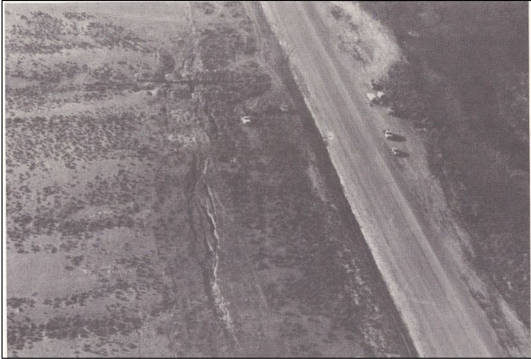
Figure 6-4. Aerial photograph showing the 1985 Whiskey Springs investigation site and lateral spread effects, left to right in this view is east to west (Andrus et al. 1987).
