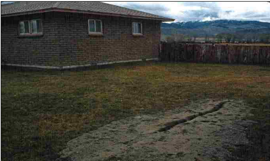
Figure 5-2. Photograph showing sand and gravel ejecta that erupted through a fissure in the ground at Pence Ranch after the M_w 7.3 Borah Peak Earthquake in 1983 (Youd et al. 1985).
